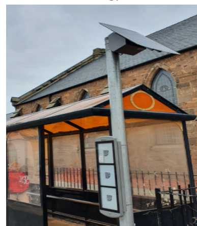
Figure 22. E-ink timetable display with solar energy source
